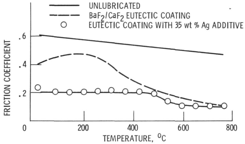
Figure 3. - Effect of silver addition to BaF<sub>2</sub>/CaF<sub>2</sub> furnace-fused coating.
