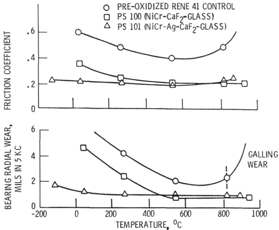
Figure 5. - Effect of silver addition on the friction and wear of plasma-sprayed, nichrome-matrix coatings (from Ref. 12). Lubricating plain spherical bearings at a radial load of 34 MPa. Bearing material, precipitation hardened nickel-chromium alloy.
