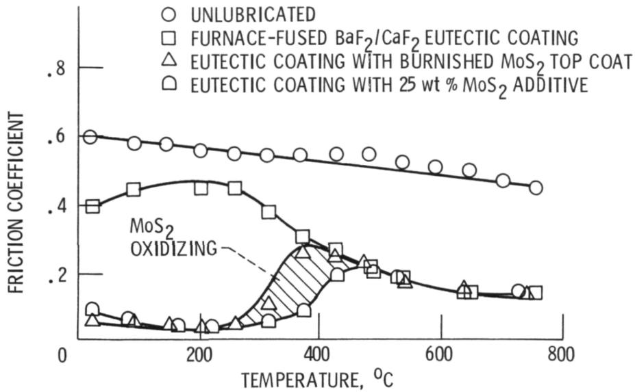
Figure 1. - Effect of MoS<sub>2</sub> as a burnished top coat and as an additive to BaF<sub>2</sub>/CaF<sub>2</sub> eutectic furnace-fused coatings. Dry air atmosphere, 2, 3 m/s, 500-gram load cast Inconel rider, Inconel 750 disks with 0.004 cm coatings.
