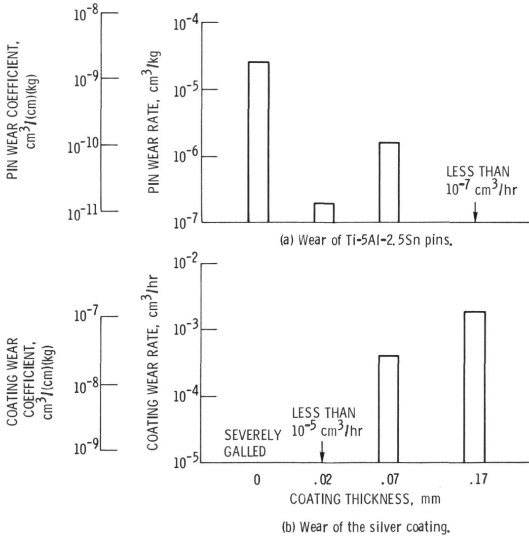
Figure 11. - Effect of silver coating thickness on pin and coating wear in air.
