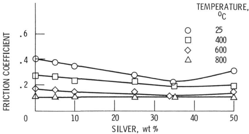
Figure 2. - Optimization of silver content in furnace-fused BaF<sub>2</sub>/CaF<sub>2</sub> eutectic coatings.
