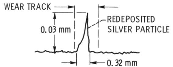
(d) 0.02-Millimeter coating; 6.9-hour duration (built up area).
