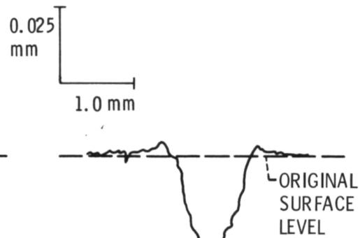
(b) 0.07-Millimeter coating; 6.5-hour duration.
