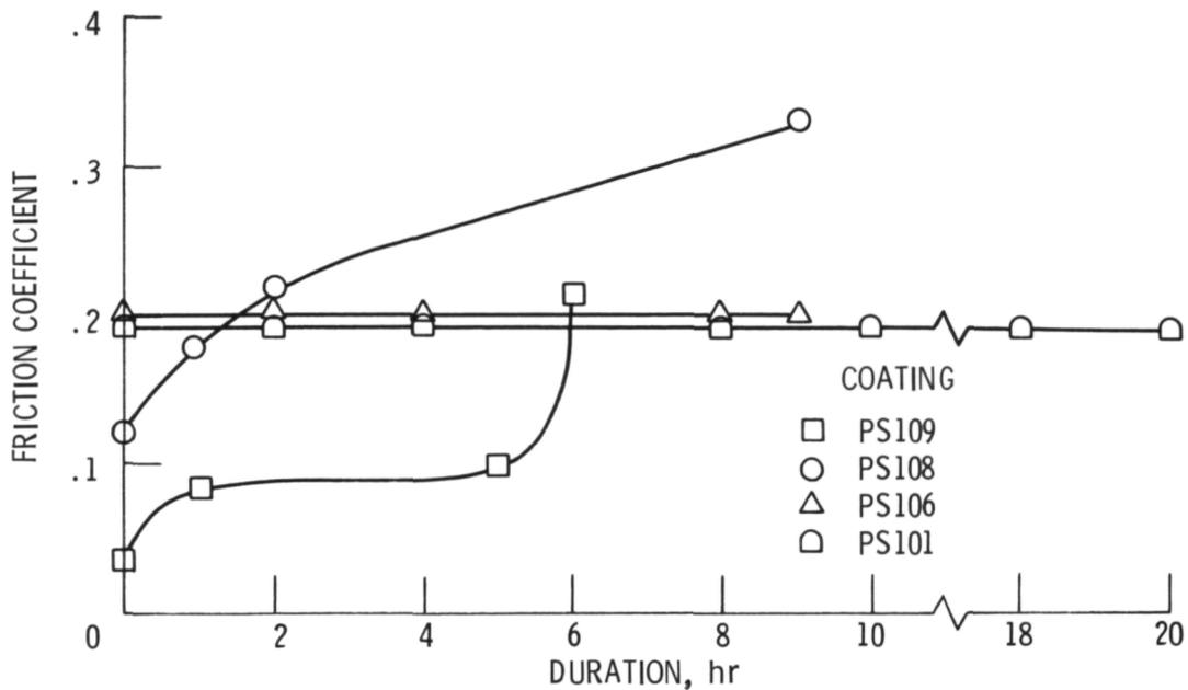
Figure 6. - Friction characteristics in air of 0.17-millimeter-thick plasma-sprayed composite coatings containing silver. Ti-5Al-2.5Sn pin material; 430 °C; 250-gram load; 13-centimeter-per-second sliding velocity at 50 rpm.
