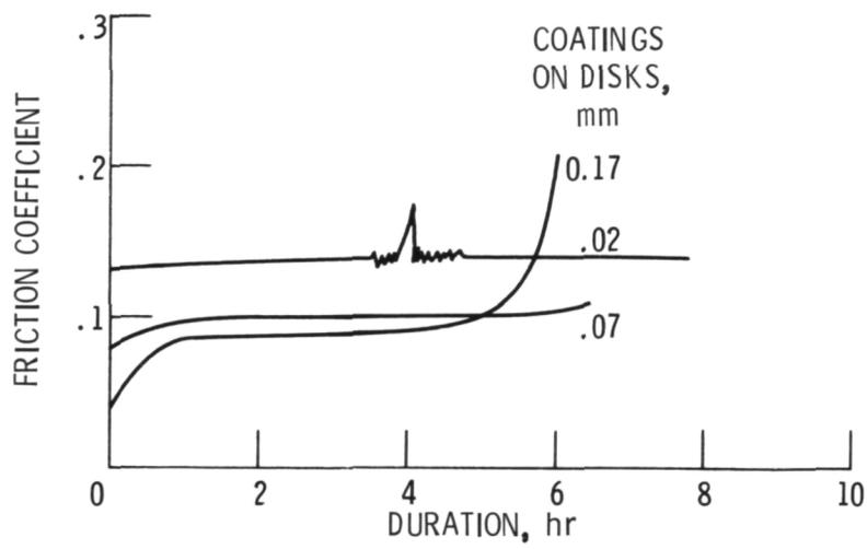
Figure 9. - Effect of coating thickness on friction of plasma-sprayed silver in air.
