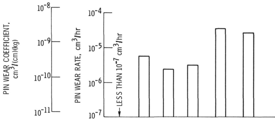
(a) Wear of Ti-5Al-2.5Sn pins.
