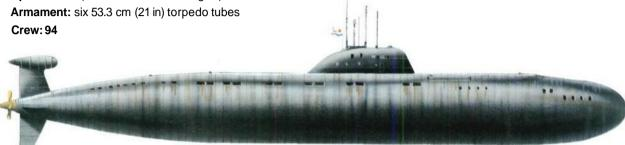
**Above:** The most distinctive feature of the Russian 'Victor III' nuclear attack submarine is the teardrop-shaped pod on top of the upper rudder housing a towed array sonar.
