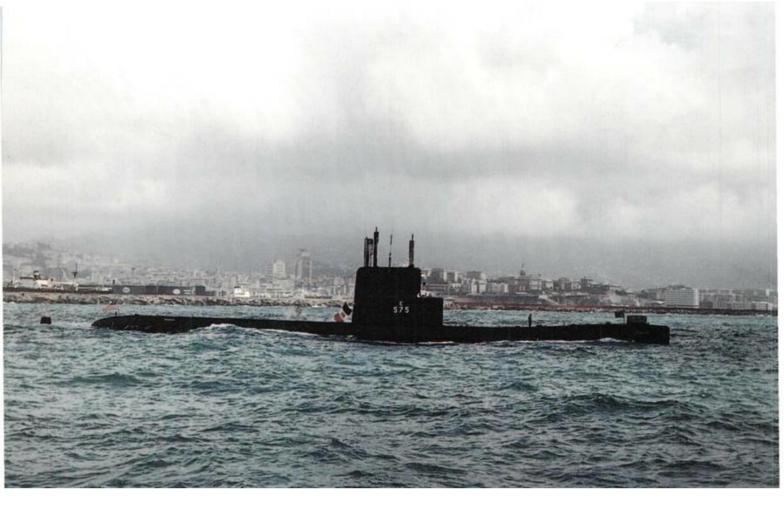
**Above:** The USS *Seawolfwas* the second prototype SIM in the US Navy, using the S2G sodium-cooled reactor. She was later re-engined with a pressurised water S2Wa plant.
