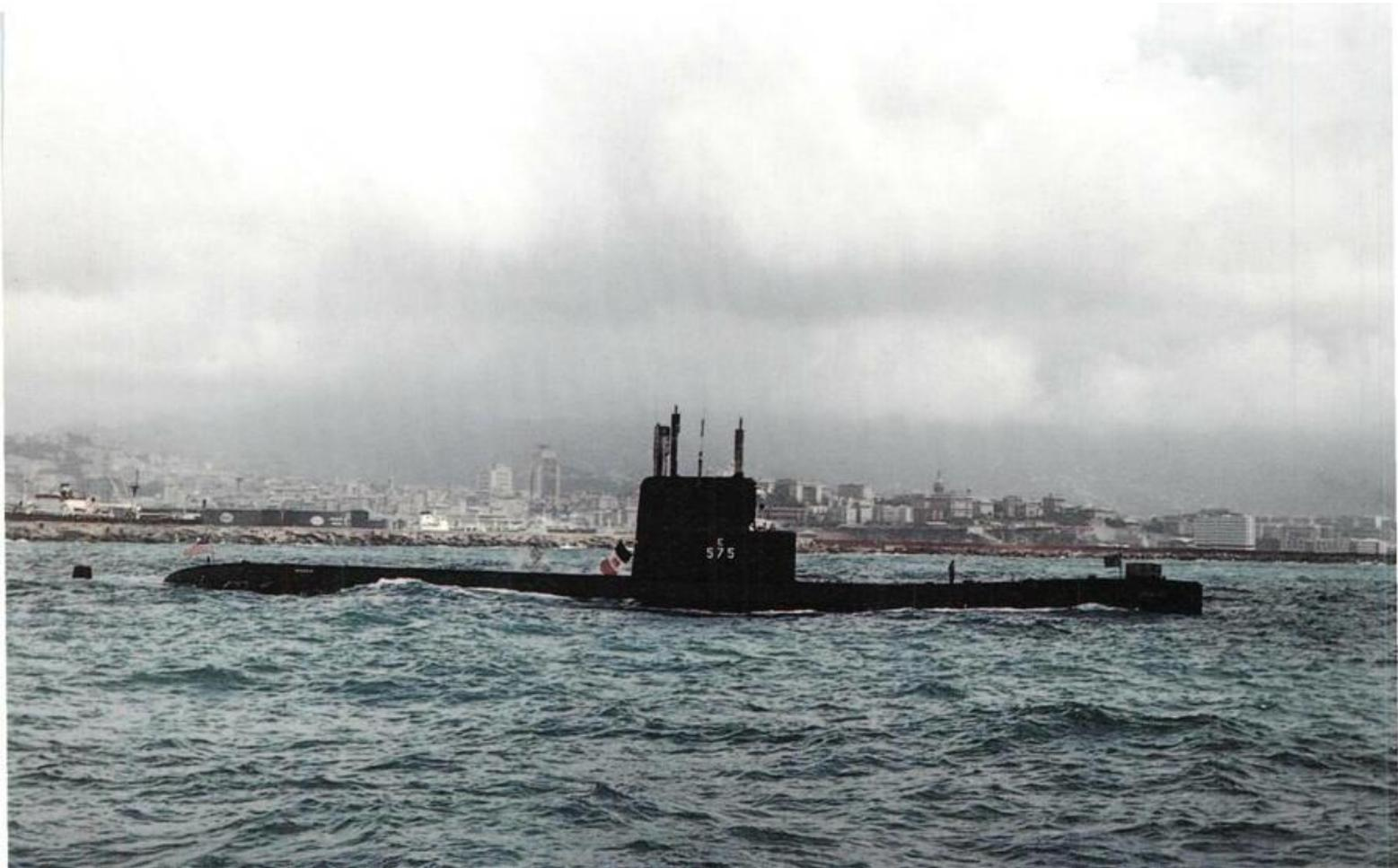
**Above:** The USS *Seawolf* was the second prototype SIM in the US Navy, using the S2G sodium-cooled reactor. She was later re-engined with a pressurised water S2Wa plant.
