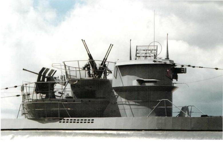
**Above:** The massive anti-aircraft armament (one 37mm and two twin 20mm guns) and radar 'mattress' give some idea of the wartime additions to the Type VII boats.
