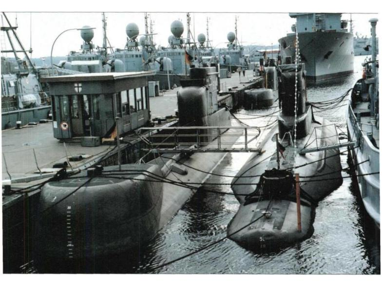
**Above:** Two Type 206A submarines at Kiel in 1995. Some 18 were built in 1971-74 and armed with DM2A1 Seeschlange wire-guided torpedoes, plus DBQS-21D sonar in the bow.
