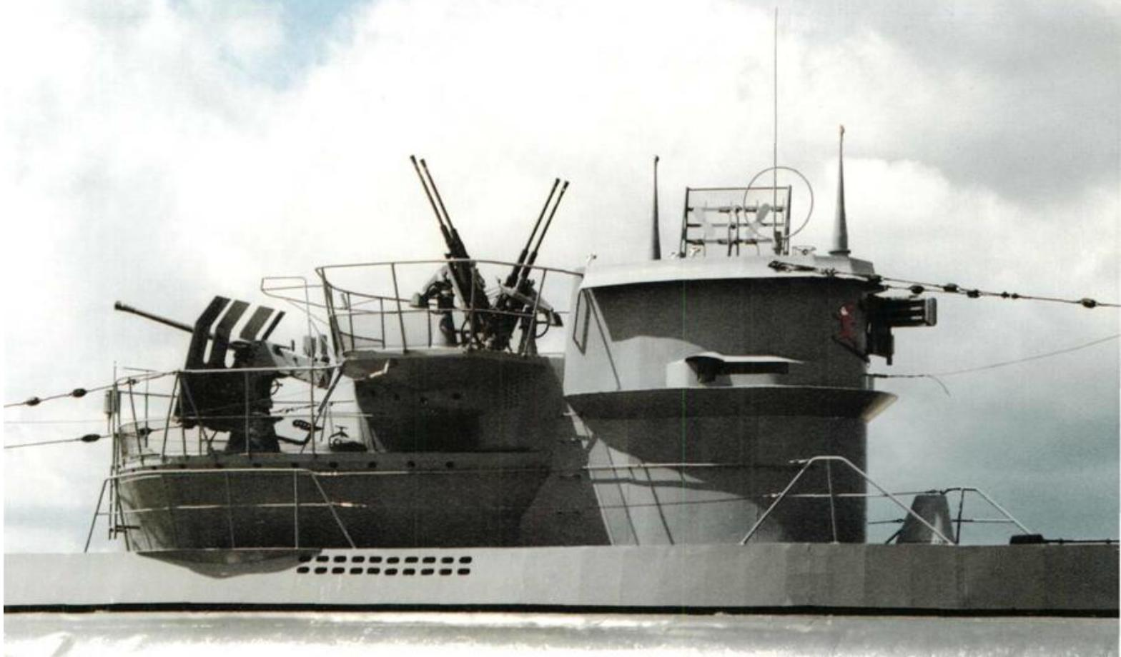
**Above:** The massive anti-aircraft armament (one 37mm and two twin 20mm guns) and radar 'mattress' give some idea of the wartime additions to the Type VII boats.
