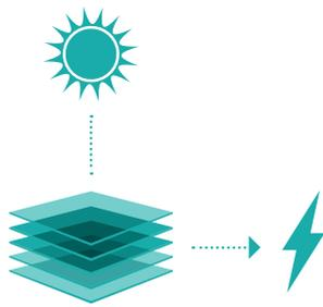
Tandem Solar Cells offer the promise of an efficiency boost, by stacking two solar cells, one on top of the other, to make the most of the available sunlight and deliver more power per unit area.
